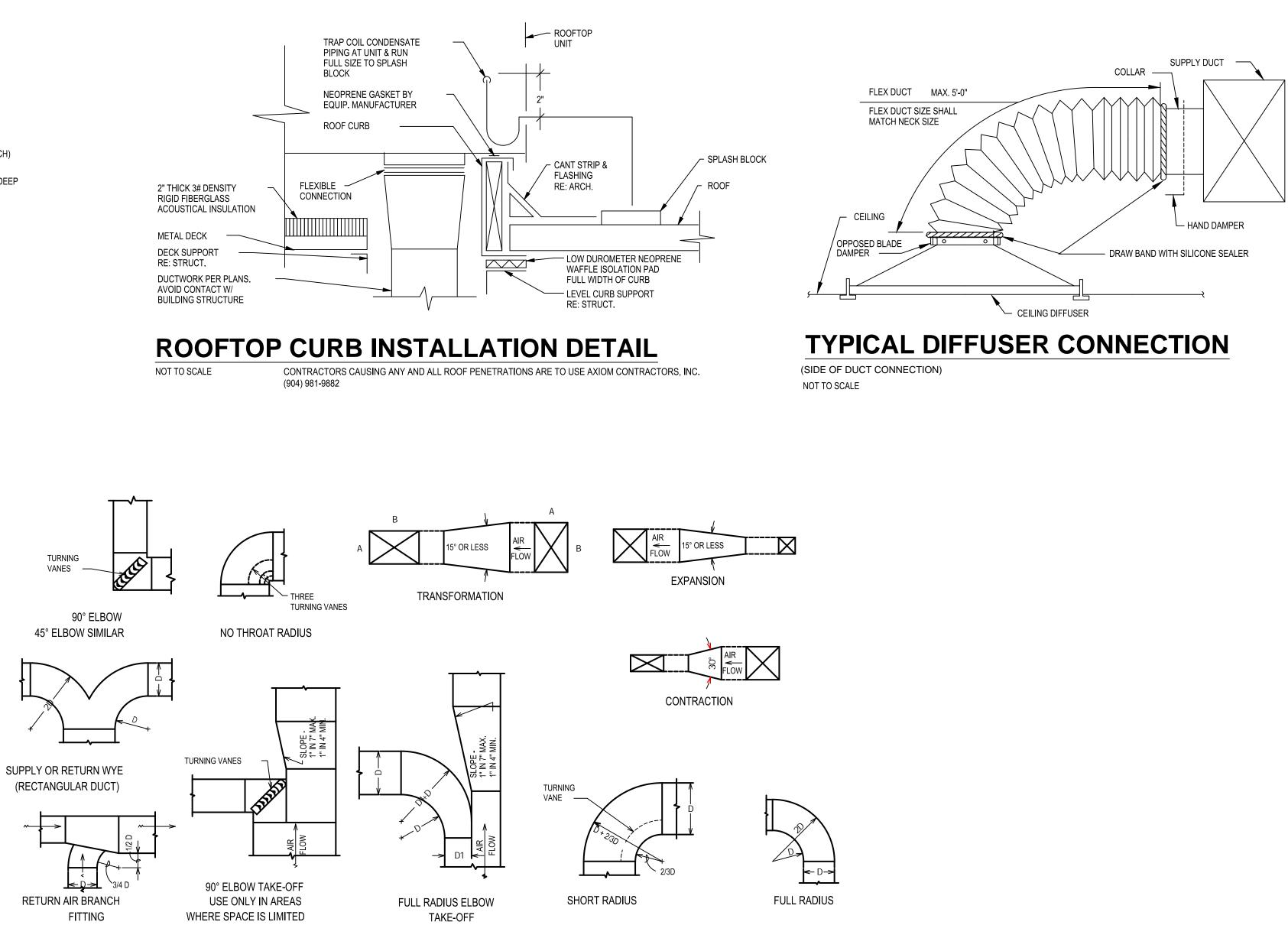
DETAILS OF THE LOW VELOCITY DUCT LAYOUT
