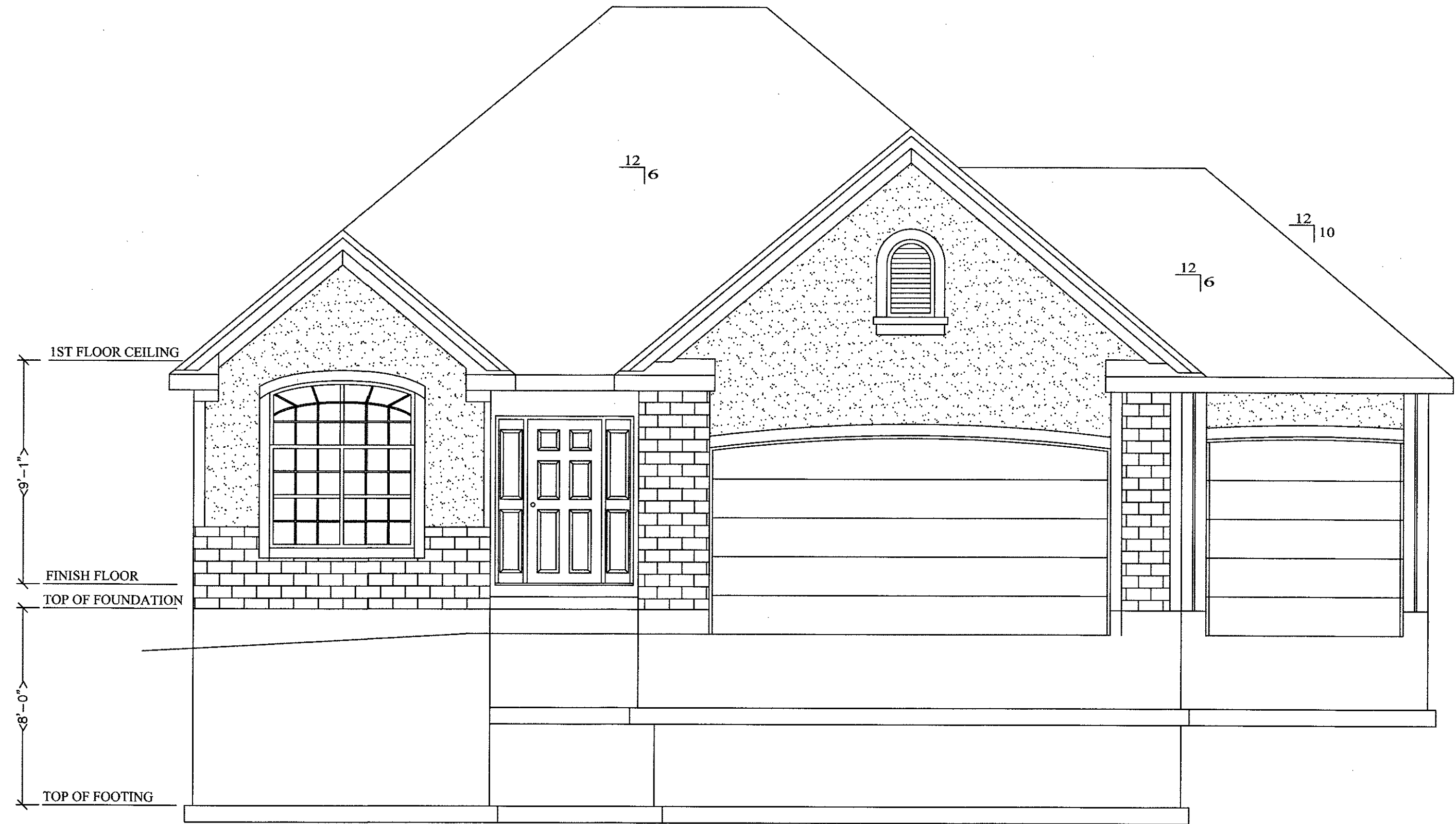
FRONT ELEVATION SCALE: 1/4" = 1'-0"
