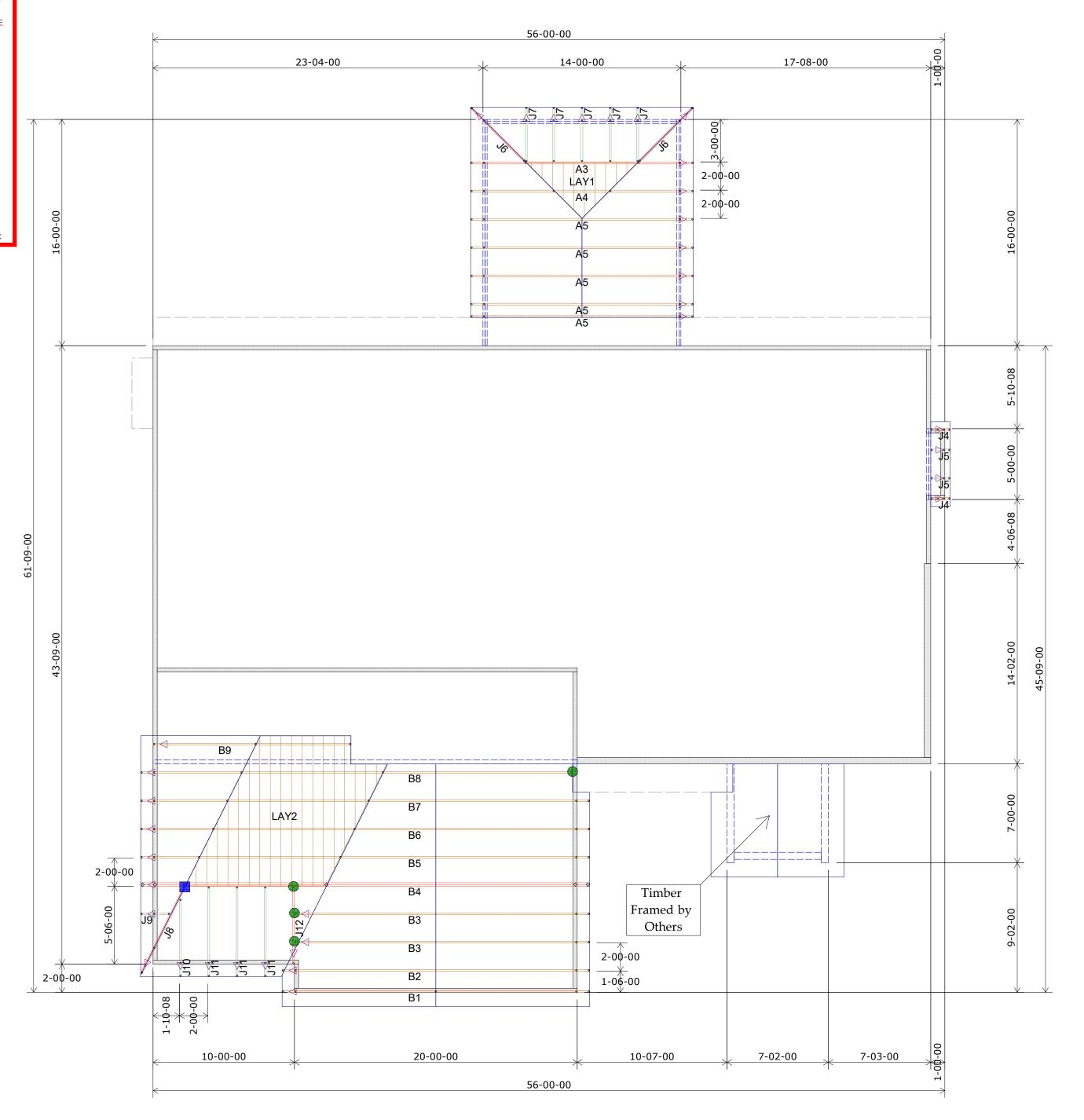
1st Floor Truss Layout Scale: 3/16" = 1'
