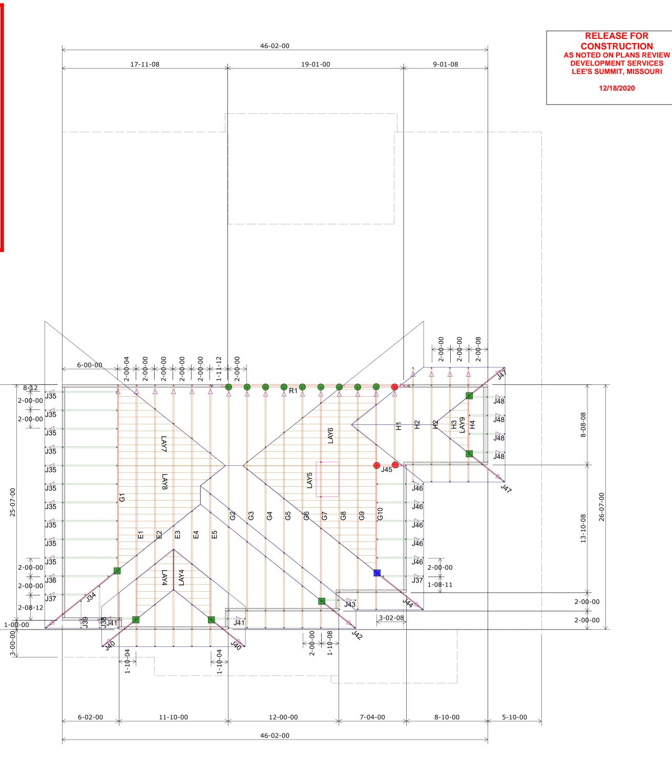
2nd Floor Truss Layout Scale: 3/16" = 1'
