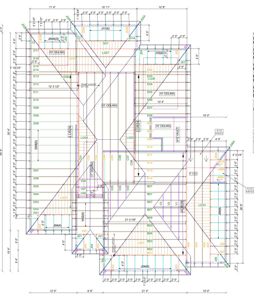
TOP TO BOTTOM PITCH 4.5/12 SOFFIT DESIGNED FOR 12" HEEL HEIGHT 7-1/4"
