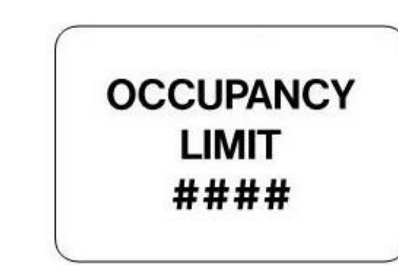
J OCCUPANCY SIGN 12" W X 6" H X 1/4" D AND 1" HELVETICA - PROVIDE AS REQUIRED BY CODE
