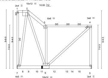
LUMBER MUST BE CUT CLEANLY AND ACCURATELY AND THE REMAINING WOOD MUST BE UNDAMAGED NO LUMBER DEFECTS ARE TO BE LOCATED WITHIN +/- 12" OF NOTCH
