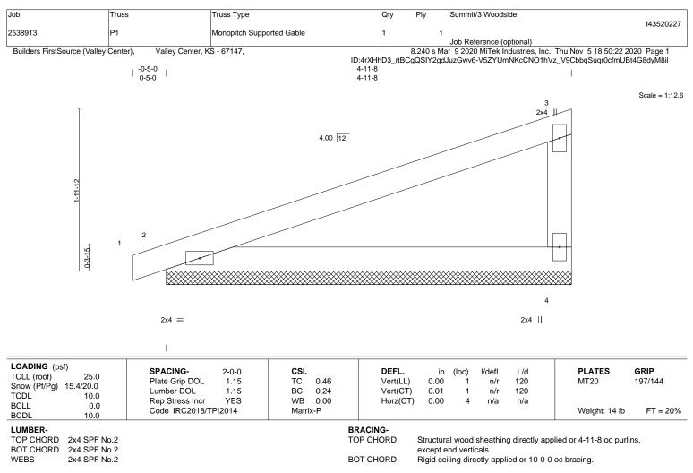
REACTIONS. (size) 4=4-11-8, 2=4-11-8 Max Horz 2=58(LC 15) Max Uplift 4=-18(LC 16), 2=-29(LC 16) Max Grav 4=226(LC 21), 2=260(LC 21)
