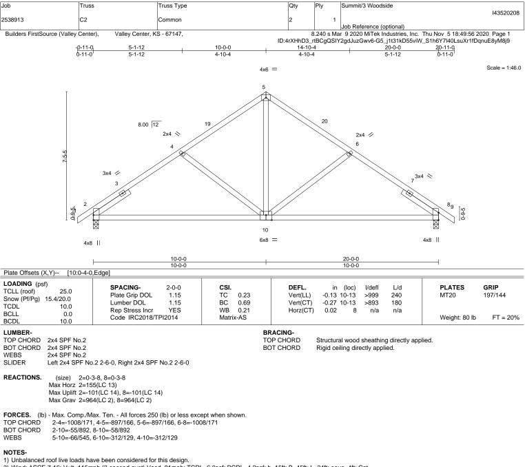
2) Wind: ASCE 7-16; Vult=115mph (3-second gust) Vasd=91mph; TCDL=6.0psf; BCDL=4.2psf; h=15ft; B=45ft; L=24ft; eave=4ft; Cat. II; Exp C; Enclosed; MWFRS (directional) and C-C Exterior(2E) -0-11-0 to 2-1-0, Interior(1) 2-1-0 to 10-0-0, Exterior(2R) 10-0-0 to 13-0-0, Interior(1) 13-0-0 to 20-11-0 zone; cantilever left and right exposed; end vertical left and right exposed; C-C for members and forces & MWFRS for reactions shown; Lumber DOL=1.60 plate grip DOL=1.60
