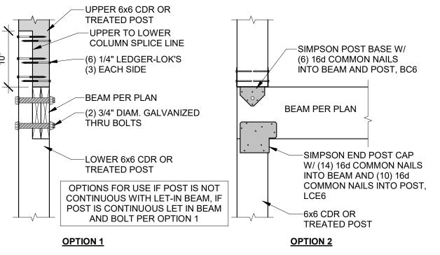
DECK LEVEL EXTERIOR BEAM TO COLUMN
