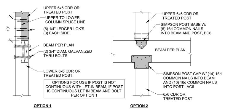
DECK LEVEL INTERIOR BEAM TO COLUMN
