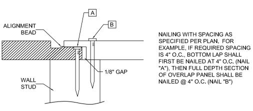
3/8" APA REQUIRED NAILING PATTERN FOR SHIPLAP PANEL SHEATHING
