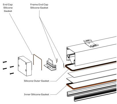
Lens and enclosure are sealed with inner and outer silicone gaskets
