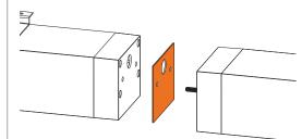
All individual sections are joined together onsite using the ¼"-20 screws and nuts provided. The joint between 2 adjacent individual sections is sealed by a silicone gasket attached to one of the 2 sections. The electrical connection between sections is made through the holes provided in the end-caps.
