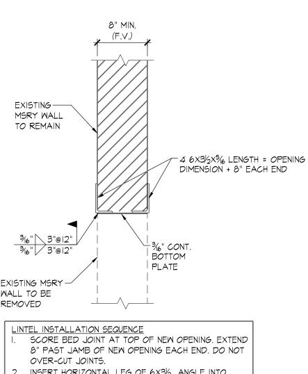
INSERT HORIZONTAL LEG OF 6X31/2 ANGLE INTO SCORED BED JOINT REPEAT STEPS | & 2 FOR OPPOSITE SIDE OF WALL
