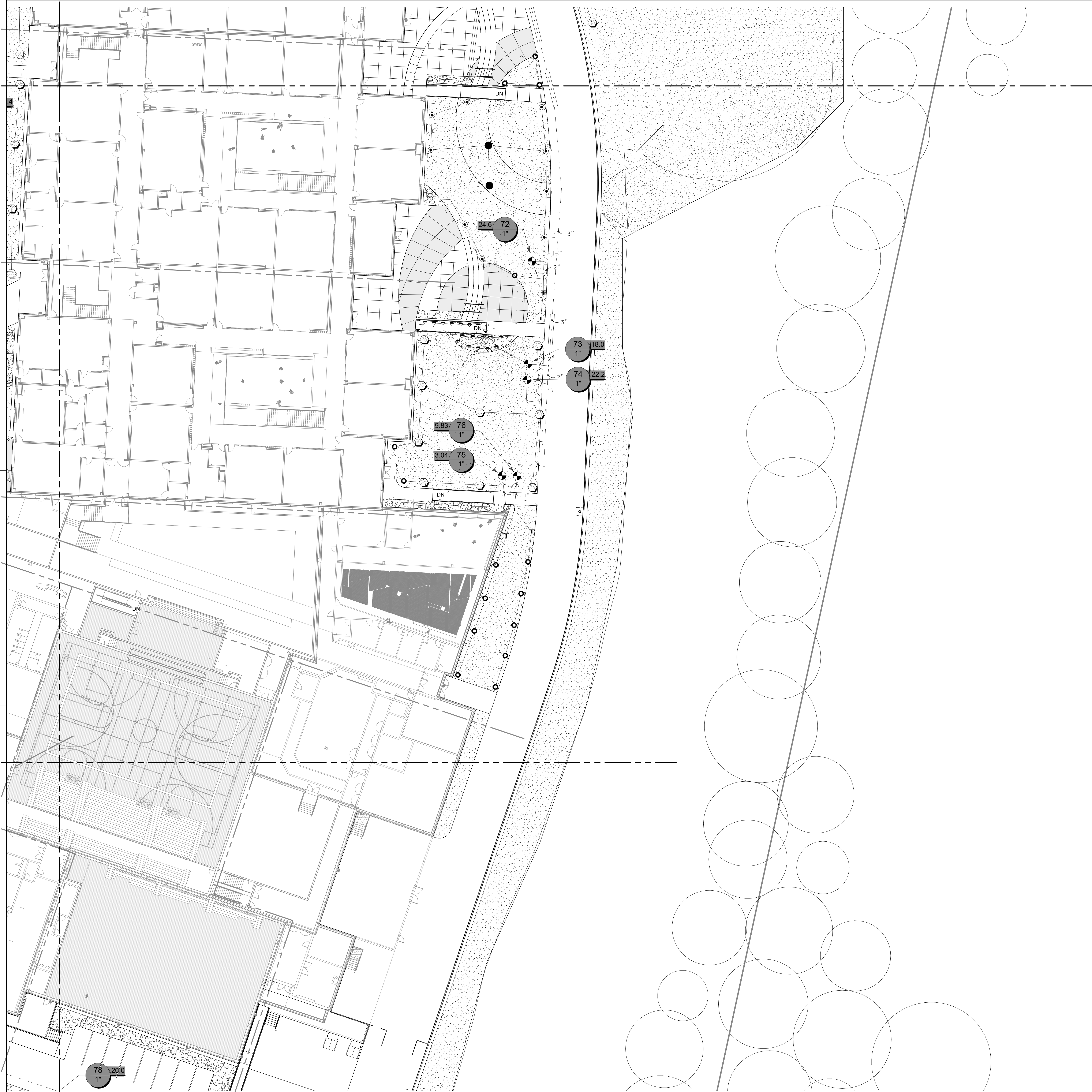
1 CD - ENLARGED IRRIGATION PLAN - BACKYARD L3.6 SCALE: 1" = 20'-0"
