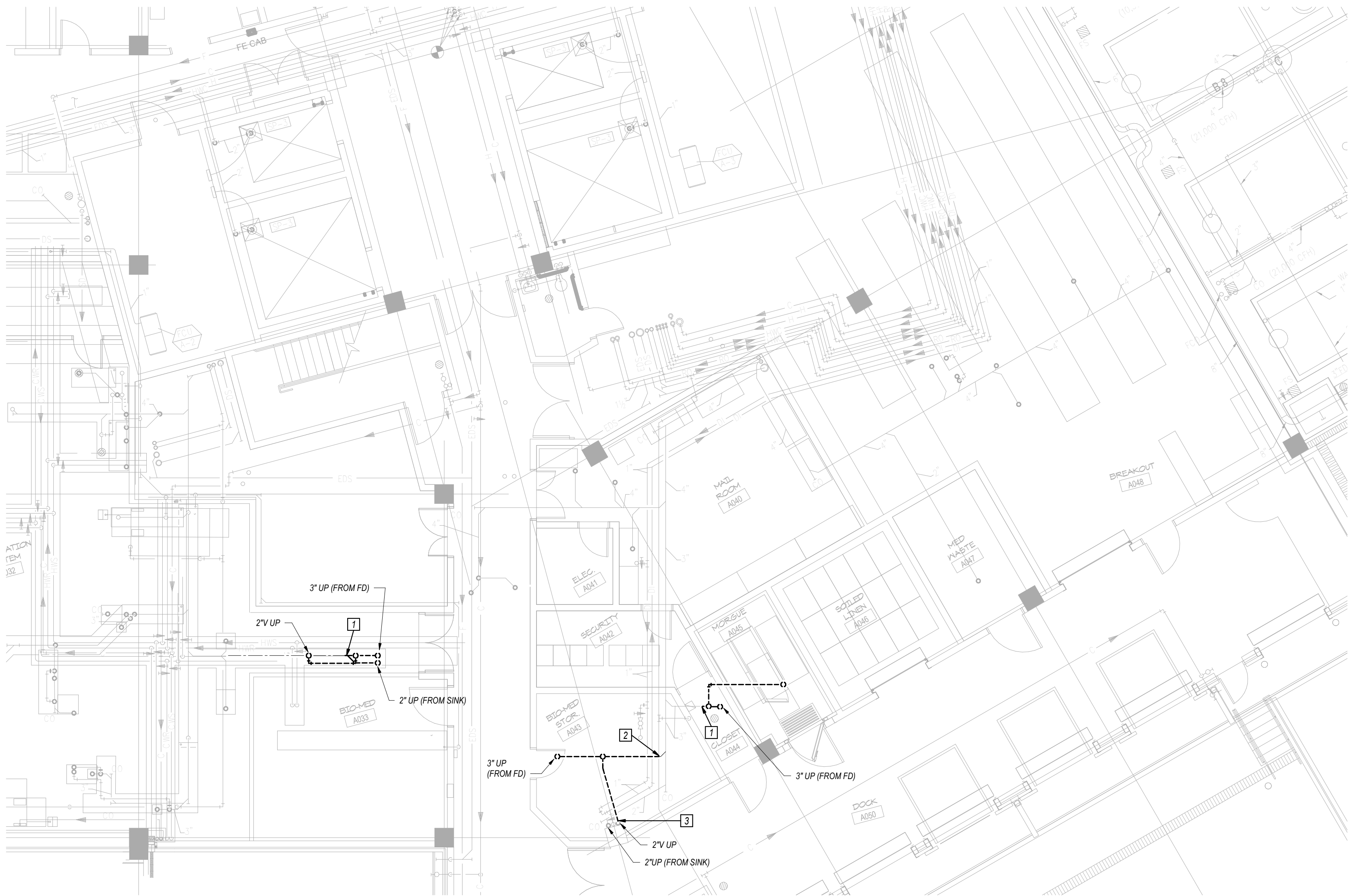
1 BASEMENT PLUMBING DEMOLITION PLAN 1/8" = 1'-0"
