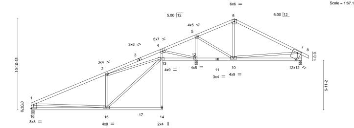
15-8-0 19-7-12 8-11-7 4-6-9 Plate Offsets (X,Y)--[6:0-2-12,Edge], [9:0-4-12,0-2-12], [16:Edge,0-5-11] GRIP LOADING (psf) SPACING-DEFL. (loc) I/defI L/d **PLATES TCLL** 25.0 Plate Grip DOL 1.15 TC 0.88 Vert(LL) -0.15 15-16 >999 360 MT20 197/144 **TCDL** 10.0 Lumber DOL 1.15 ВС 0.58 Vert(CT) -0.31 15-16 >766 240 **BCLL** 0.0 Rep Stress Incr YES WB 0.88 Horz(CT) 0.03 12 n/a n/a Code IRC2018/TPI2014 Wind(LL) FT = 10% BCDL 10.0 Matrix-S 0.04 >999 240 Weight: 127 lb 15
