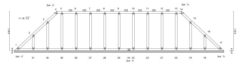
Plate Offsets (X,Y)--[4:0-1-10,Edge], [14:0-1-10,Edge] GRIP LOADING (psf) SPACING-CSI. DEFL. in (loc) I/defI L/d **PLATES TCLL** 25.0 Plate Grip DOL 1.15 TC 0.06 Vert(LL) 999 MT20 197/144 n/a n/a **TCDL** 10.0 Lumber DOL 1.15 ВС 0.04 Vert(CT) n/a n/a 999 **BCLL** 0.0 Rep Stress Incr YES WB 0.07 0.01 17 Horz(CT) n/a n/a Code IRC2018/TPI2014 FT = 10% BCDL Matrix-S Weight: 134 lb 10.0
