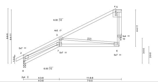
Plate Offsets (X,Y)--[2:0-2-8,0-2-8], [4:Edge,0-1-14] SPACING-DEFL. GRIP LOADING (psf) CSI. (loc) I/defI L/d **PLATES** 197/144 **TCLL** 25.0 Plate Grip DOL 1.15 TC 0.60 Vert(LL) -0.14 >985 360 MT20 **TCDL** 10.0 Lumber DOL 1.15 ВС 0.62 Vert(CT) -0.29 6-7 >475 240 M18SHS 197/144 **BCLL** 0.0 Rep Stress Incr YES WB 0.76 Horz(CT) 0.13 10 n/a n/a Code IRC2018/TPI2014 Wind(LL) **BCDL** 10.0 Matrix-S >999 240 Weight: 47 lb FT = 10% 0.10 7
