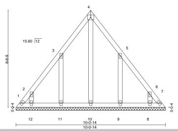
LOADING (psf) SPACING-2-0-0 CSI. DEFL. I/defI L/d **PLATES** GRIP (loc) TCLL 25.0 Plate Grip DOL 1.15 Vert(LL) 197/144 TC 0.06 n/a n/a 999 MT20 **TCDL** 10.0 Lumber DOL 1.15 ВС 0.03 Vert(CT) n/a 999 n/a **BCLL** 0.0 Rep Stress Incr YES WB 0.07 Horz(CT) 0.00 n/a n/a Code IRC2018/TPI2014 BCDL 10.0 Matrix-S Weight: 45 lb FT = 10%
