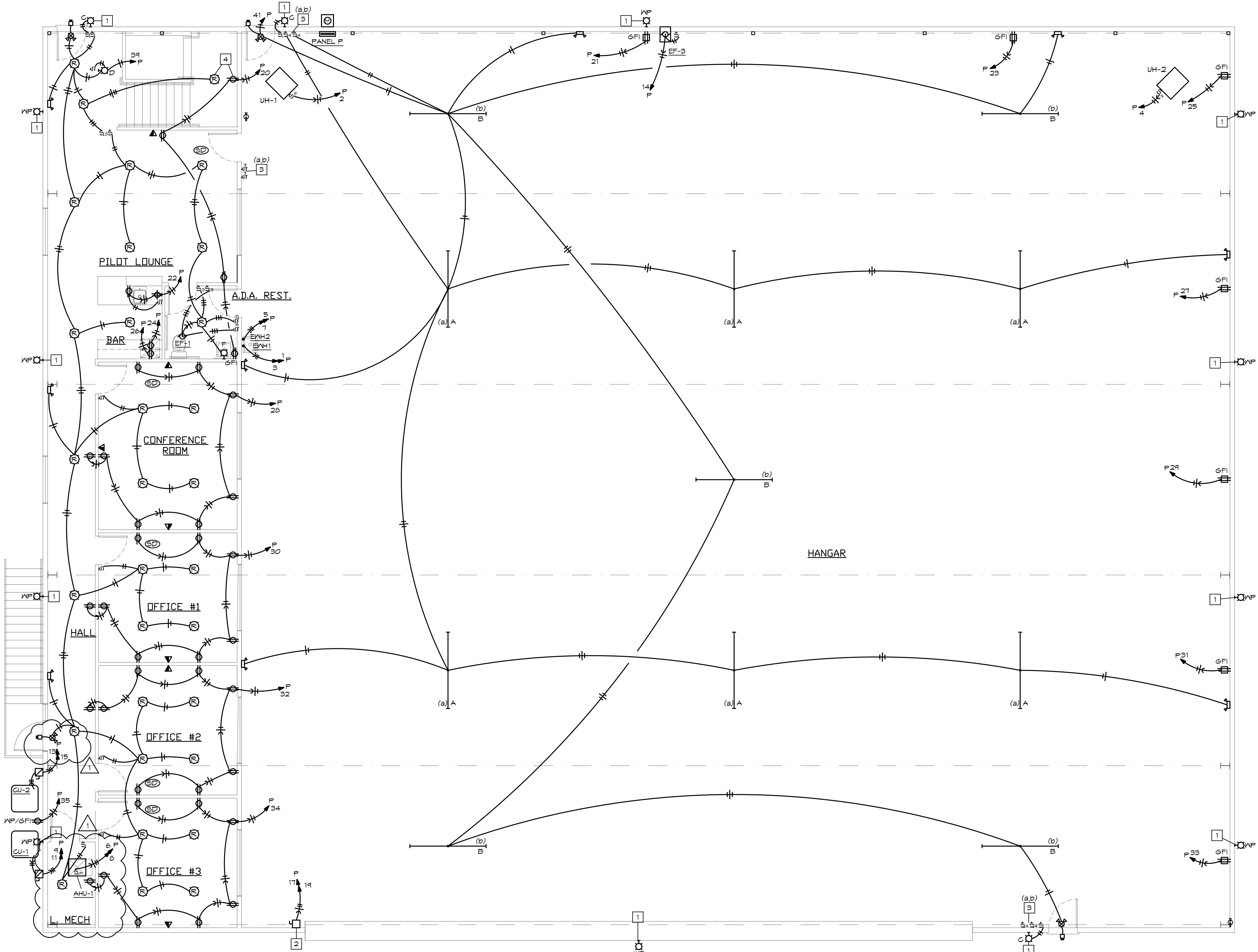
MAIN FLOOR ELECTRICAL PLAN SCALE: 3/16" = 1'-0"
