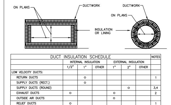
NOTES: INSULATION SHALL BE INSTALLED WHEN INDICATED OTHERWISE IN THE CONSTRUCTION DOCUMENTS. OTHERWISE, NO INSULATION IS REQUIRED.
