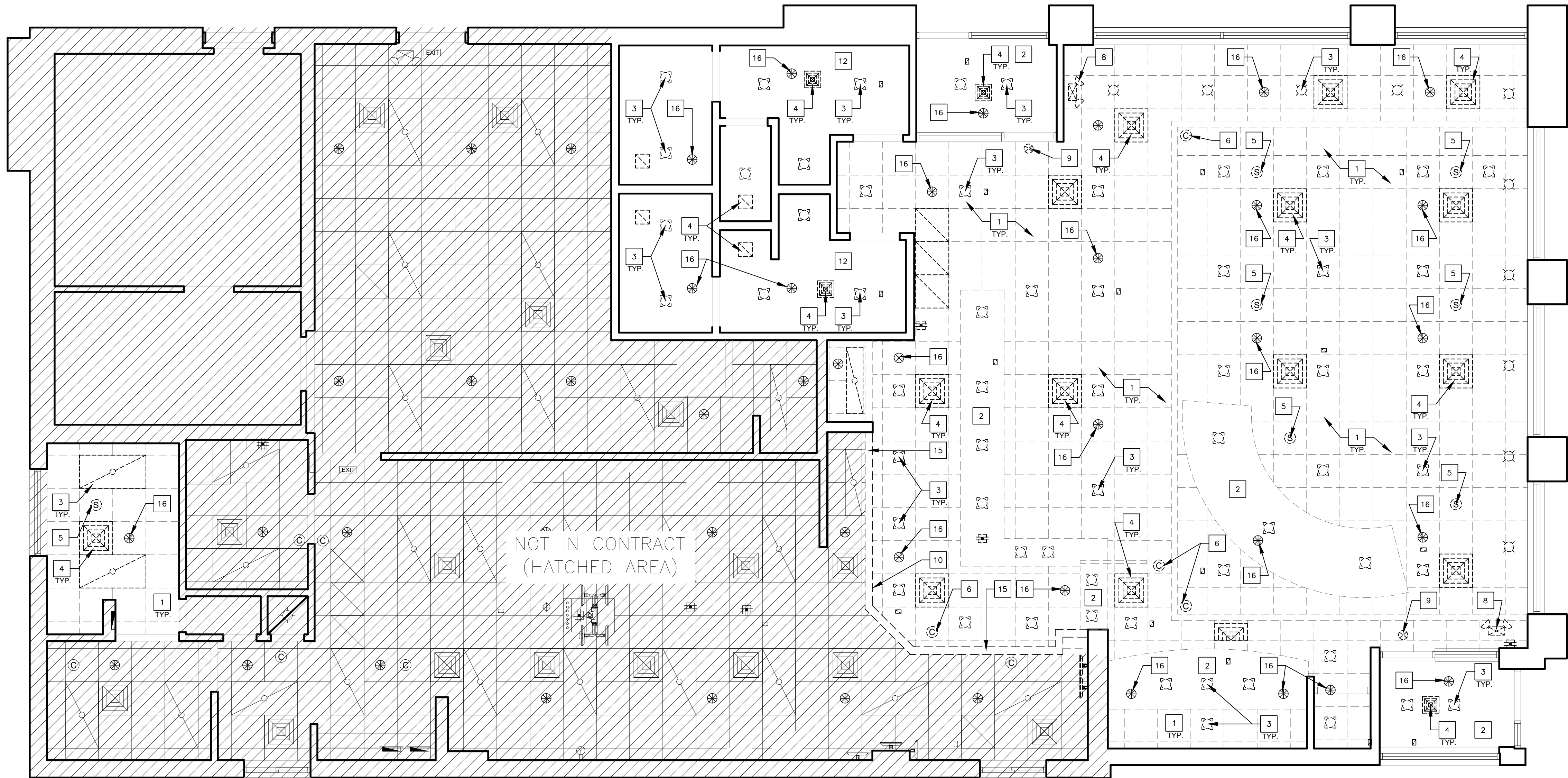
1 D1.1 DEMOLITION REFLECTED CEILING PLAN SCALE: 1/4" = 1'-0"
