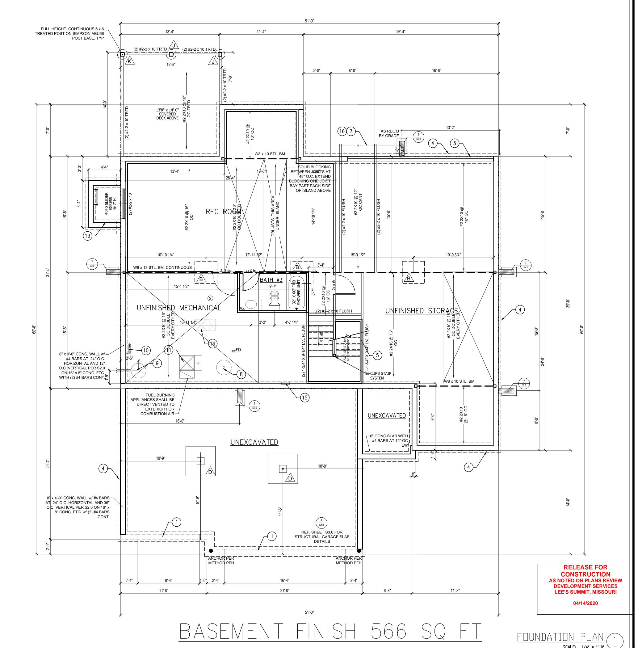
\*\*ALL INTERIOR NON-LOAD BEARING, NON-BRACED, NON-CABINET WALLS ARE ALLOWED AT 24" OC.
