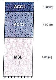
Subgrade Modulus = 5,000 (psi) Structural Number = 3.868 Calculated Traffic (ESALs) = 976,000
