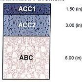
Subgrade Modulus = 27,083 (psi) Structural Number = 2.670 Calculated Traffic (ESALs) = 4,153,000
