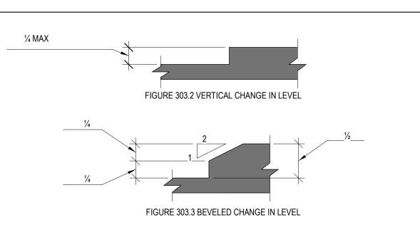
303.2 VERTICAL. CHANGES IN LEVEL OF 1/4" HIGH MAXIMUM SHALL BE PERMITTED TO BE VERTICAL. (FIG. 303.2) 303.3 BEVELED. CHANGES IN LEVEL BETWEEN 1/4" AND 1/2" HIGH MAXIMUM SHALL BE BEVELED WITH A SLOPE NOT STEEPER THAN 1:2 (FIG. 303.3) 303.4 RAMPED. CHANGES IN LEVEL GREATER THAN 1/2" SHALL BE RAMPES AND SHALL COMPLY WITH ICC/ANSI A117.1-1998 SECTION 405 AND 406.
