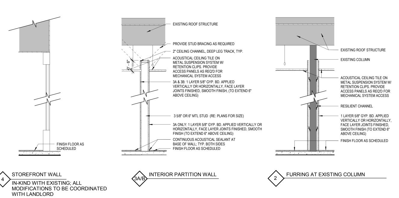
1) THE BOTTOM TRACK OF ALL PARTITIONS/WALLS SHALL BE ATTACHED TO FLOOR W/ .177 SHANK DIA. x 1 7/16" PENETRATION @ 32" O.C. POWER DRIVEN FASTENERS HILTI OR EQ. TYP. U.N.O.
