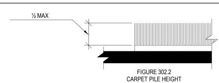
302 GENERAL. FLOOR OR GROUND SURFACES SHALL BE STABLE, FIRM AND SLIP RESISTANT, AND SHALL COMPLY WITH ICC/ANSI A117.1-1998 SECTION 302. **302.2 CARPET.** PILE HEIGHT SHALL BE 1/2" MAXIMUM. EXPOSED EDGES OF CARPET SHALL BE FASTENED TO FLOOR OR GROUND AND SHALL HAVE TRIM ALONG ENTIRE LENGTH OF EXPOSED EDGE. CARPET EDGE TRIM SHALL COMPLY WITH ICC/ANSI A117.1-1998 SECTION 303. (FIG. 302.2)
