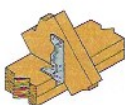
Joists to Plate with A Leg Inside
