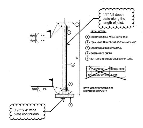
JOIST CHORD REINFORCEMENT
