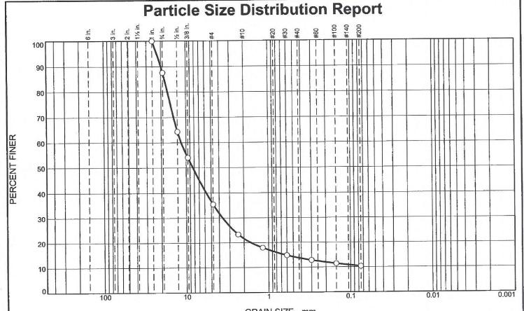
GRAIN SIZE - mm. % Fines % Gravel % Sand % +3" Silt Clay Fine Coarse Medium Fine Coarse 10 53 8 13 0 12
