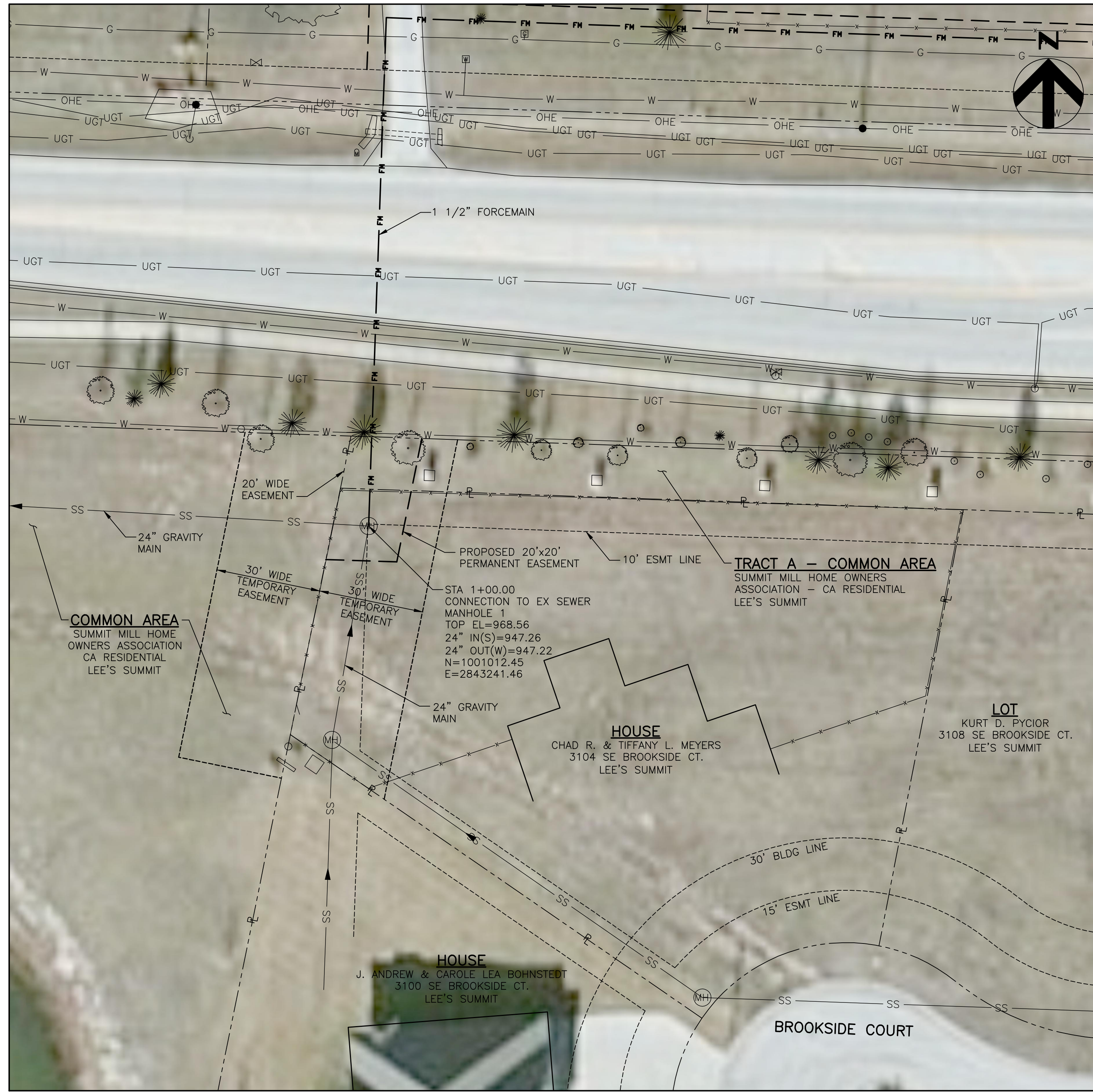
SITE PLAN - FORCEMAIN MANHOLE TIE-IN
