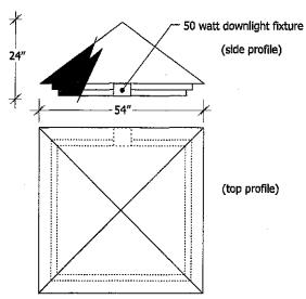
detail B - (1) 24"x54"x54" custom fabricated roof cap. Standing seam metal fabrication using 26ga. paintgrip steel.
