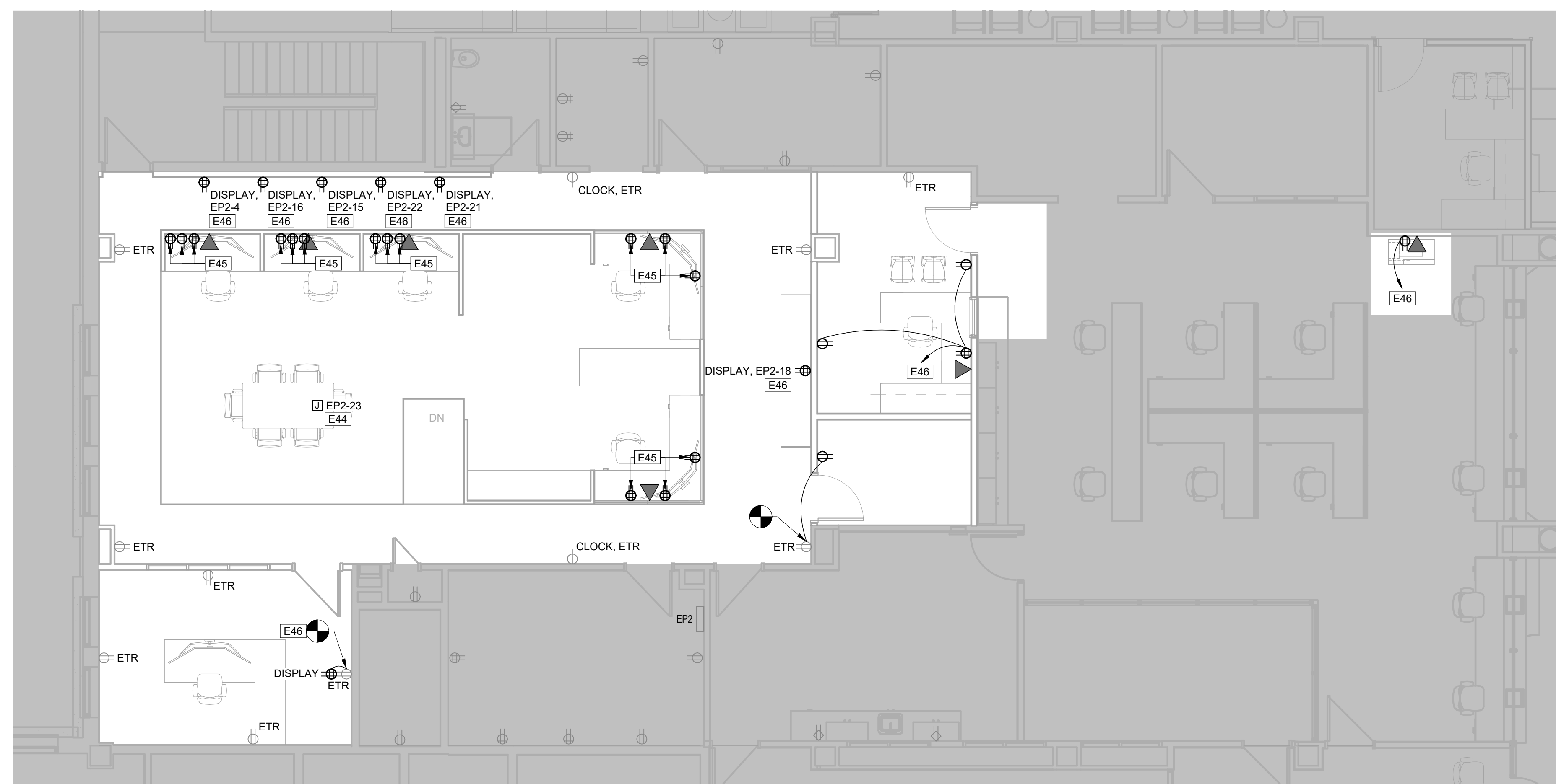
LOAD REMOVED: 12,600 VA LOAD ADDED: 8,460 VA NET CHANGE: 4,140 VA 1 REAL TIME CENTER - POWER PLAN 3/16" = 1'-0"
