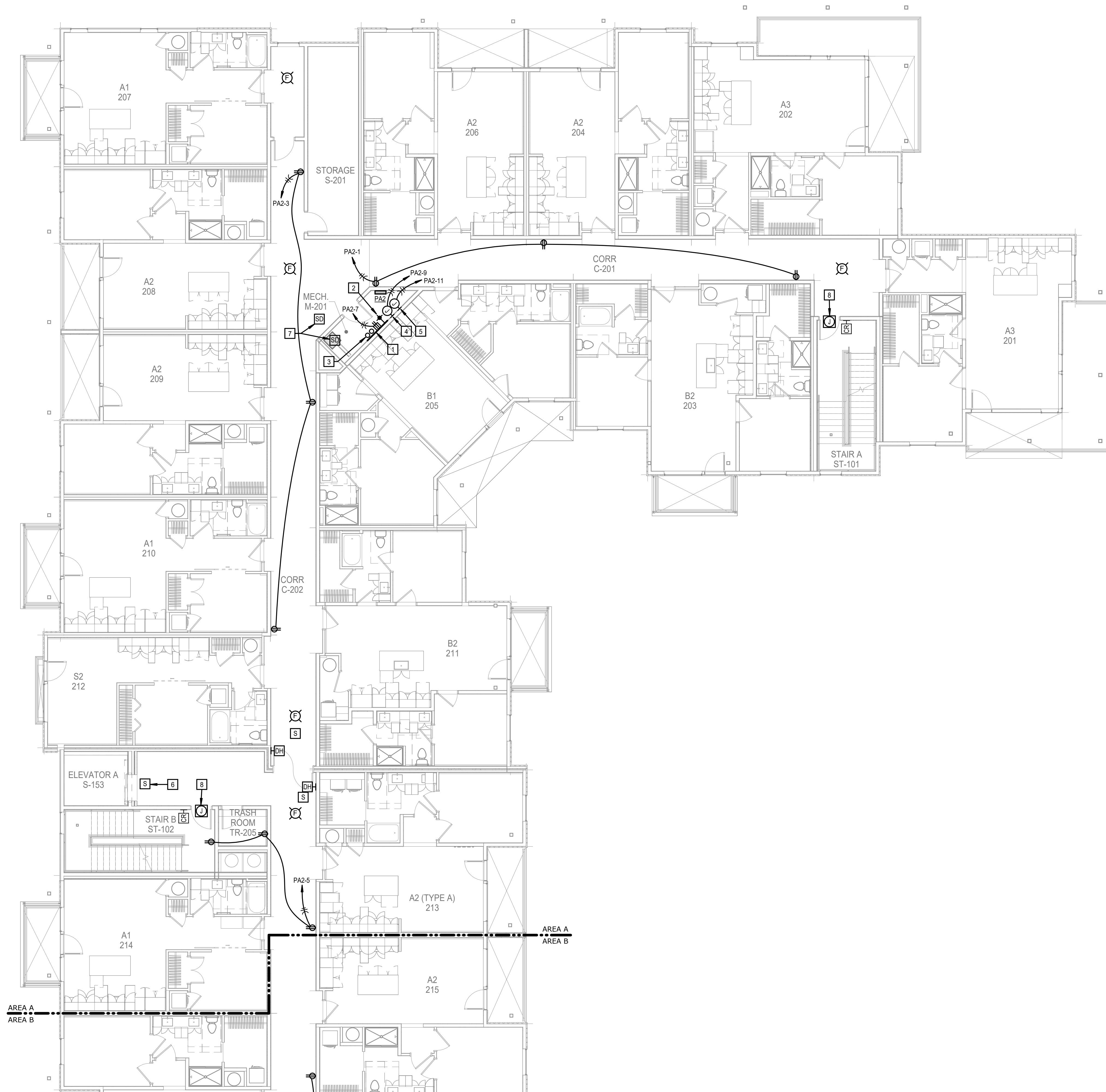
A1 SECOND FLOOR - POWER PLAN - AREA A 1/8" = 1'-0"
