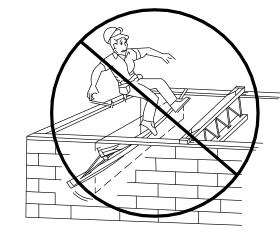
DO NOT walk on the trusses until all truss bearings and bracing have been permanently attached. Injury may result.
