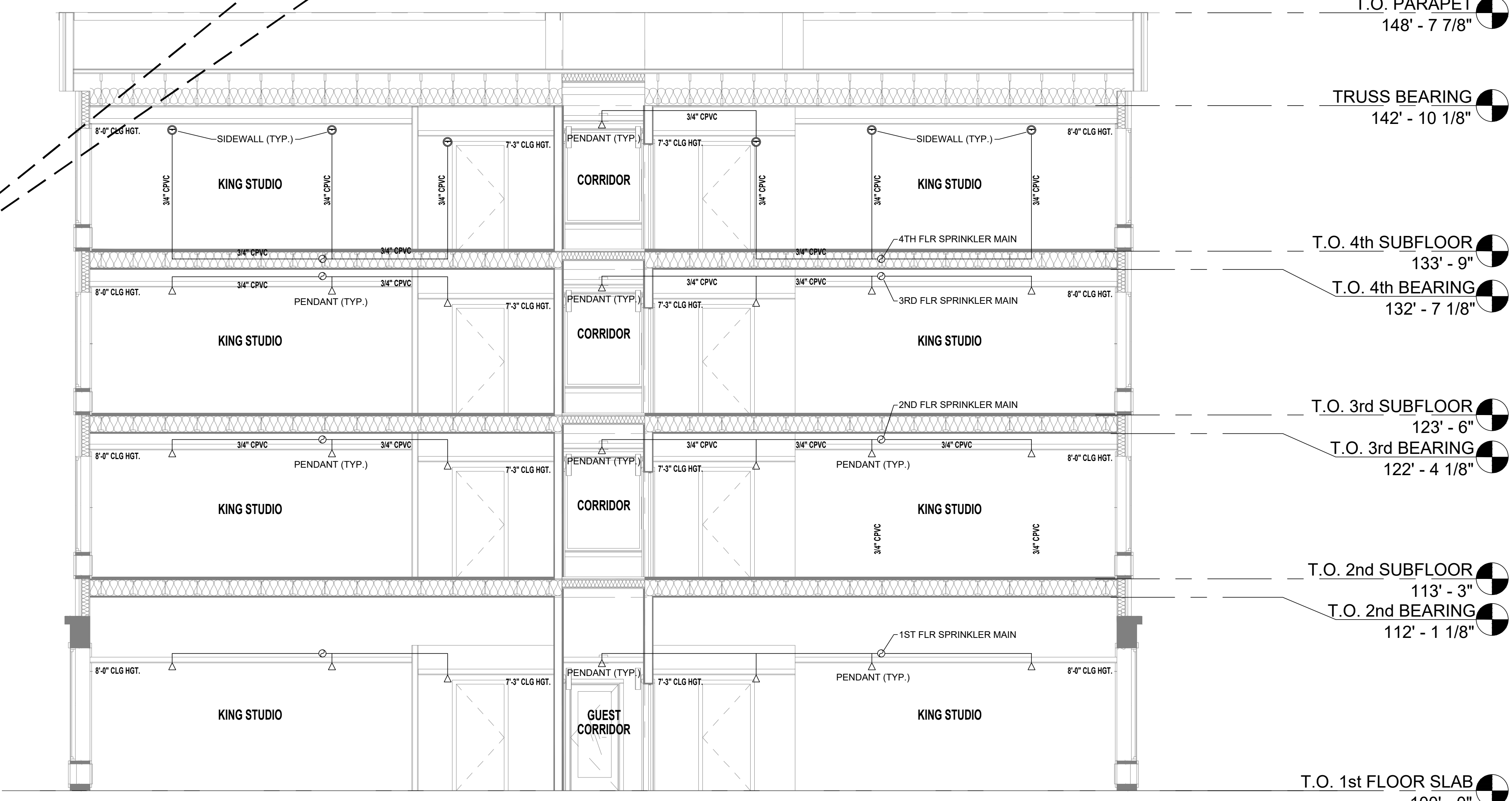
BUILDING CROSS SECTION
