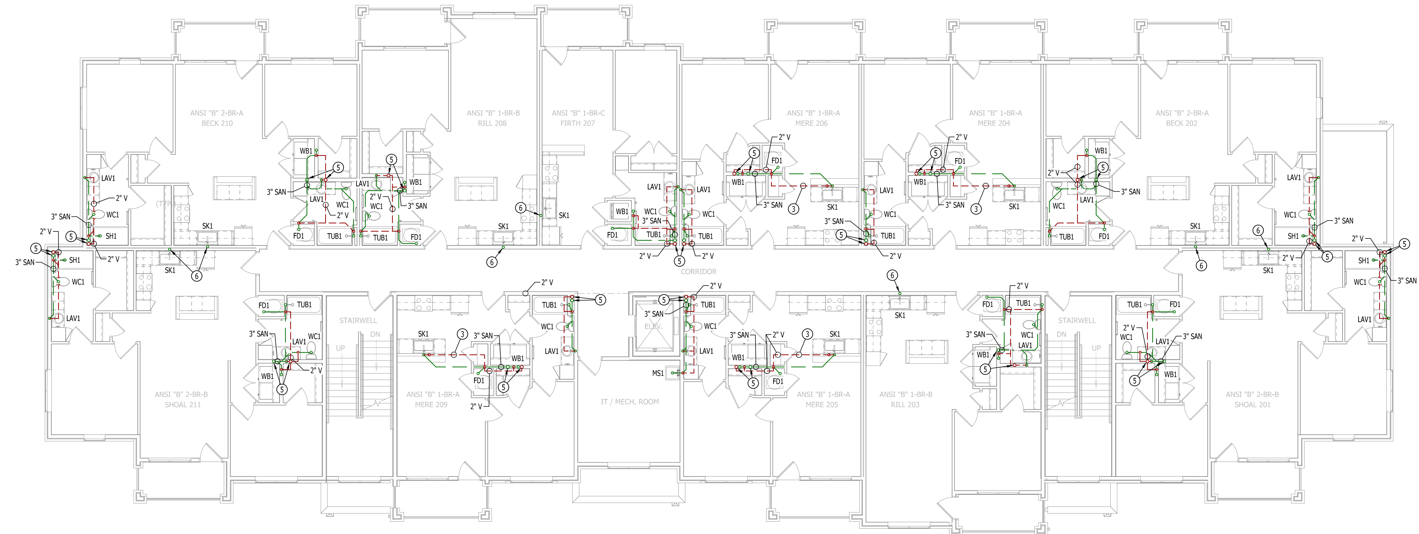
SANITARY SEWER PLAN - SECOND FLOOR SCALE: 1/8" = 1'-0"
