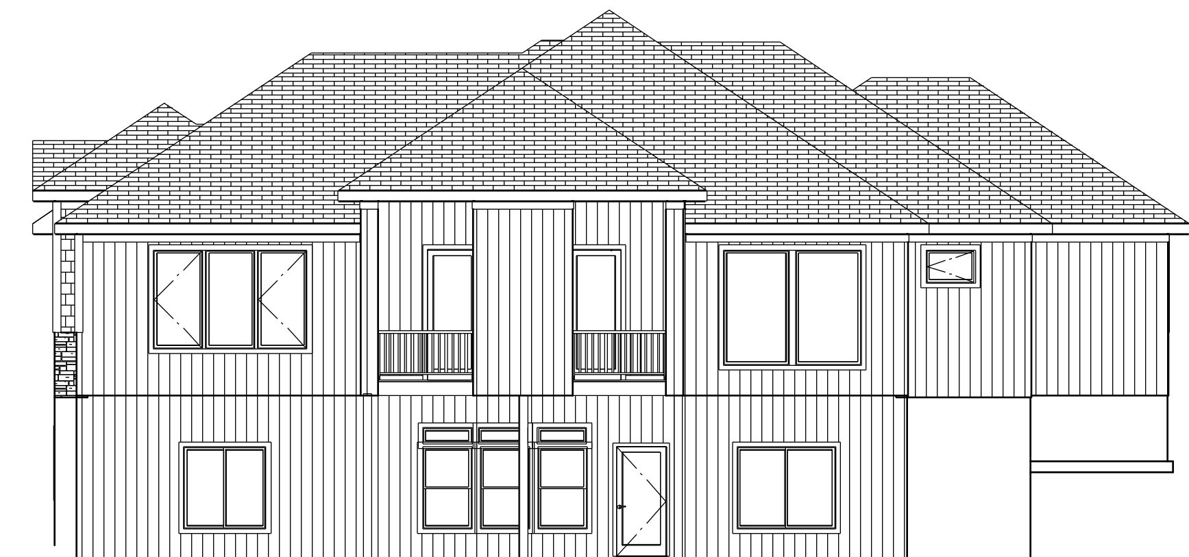
REAR EL. 1/8 = 1-0 LP SIDING PANEL SIDING
