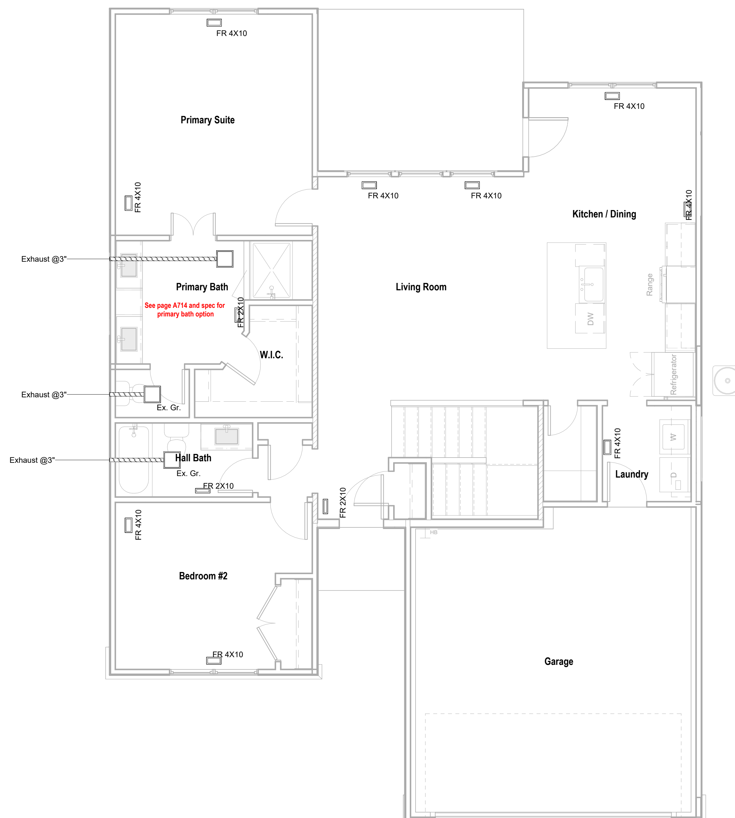
② Main Level Plan HVAC 1/4" = 1'-0"
