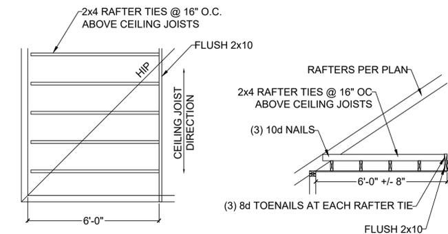
**5 RAFTER TIES AT CEILING JOISTS PERP. TO RAFTERS**
