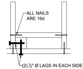
**7** ALTERNATE COVERED DECK/PORCH INTERSECTION CORNER BEAM CONNECTION
