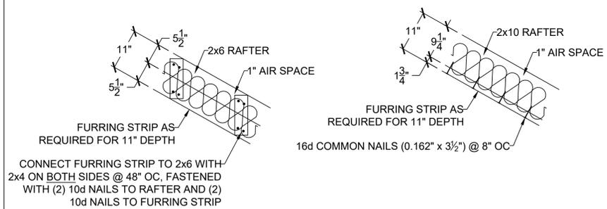
**3 VAULTED RAFTER INSULATION DETAILS**
