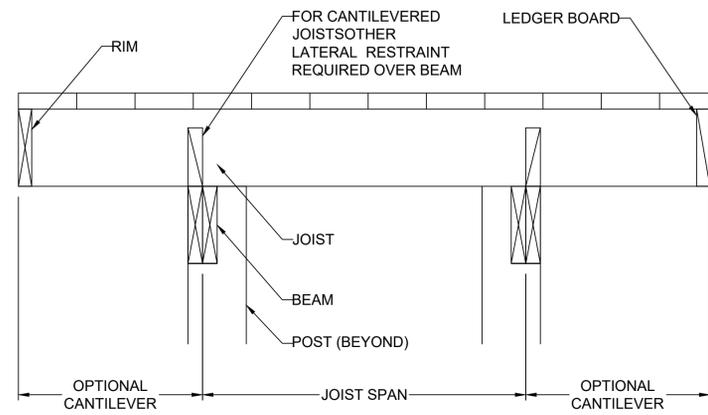
JOISTS ON FREE-STANDING DECK WITH DROPPED BEAM
