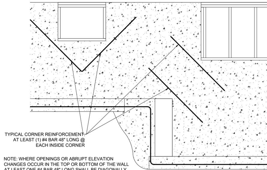
NOTE: WHERE OPENINGS OR ABRUPT ELEVATION CHANGES OCCUR IN THE TOP OR BOTTOM OF THE WALL AT LEAST ONE #4 BAR 48" LONG SHALL BE DIAGONALLY AS CLOSE AS PRACTICAL TO THE CORNER
