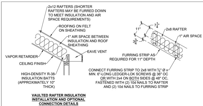
**VAULTED RAFTER INSULATION INSTALLATION AND OPTIONAL CONNECTION DETAILS**
