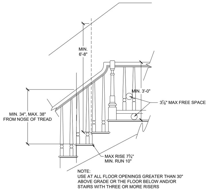
**4 STAIR AND HANDRAIL/GUARDRAIL DETAIL**
