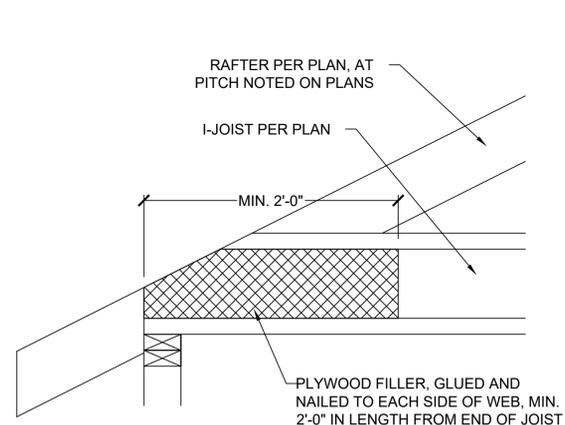
**9 COPED I-JOIST REINFORCEMENT**
