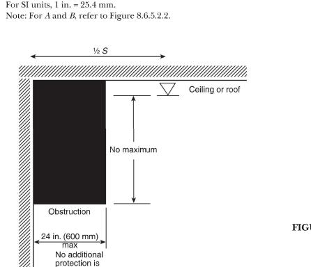
FIGURE 8.6.5.1.2(c) Obstructions Against Walls (SSU/SSP).
