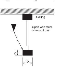
**Elevation View of Truss** (Obstruction in horizontal orientation)  $A \ge 3C \text{ or } 3D$   $A \le 24 \text{ in. (600 mm)}$ (Use dimension C or D, whichever is greater)
