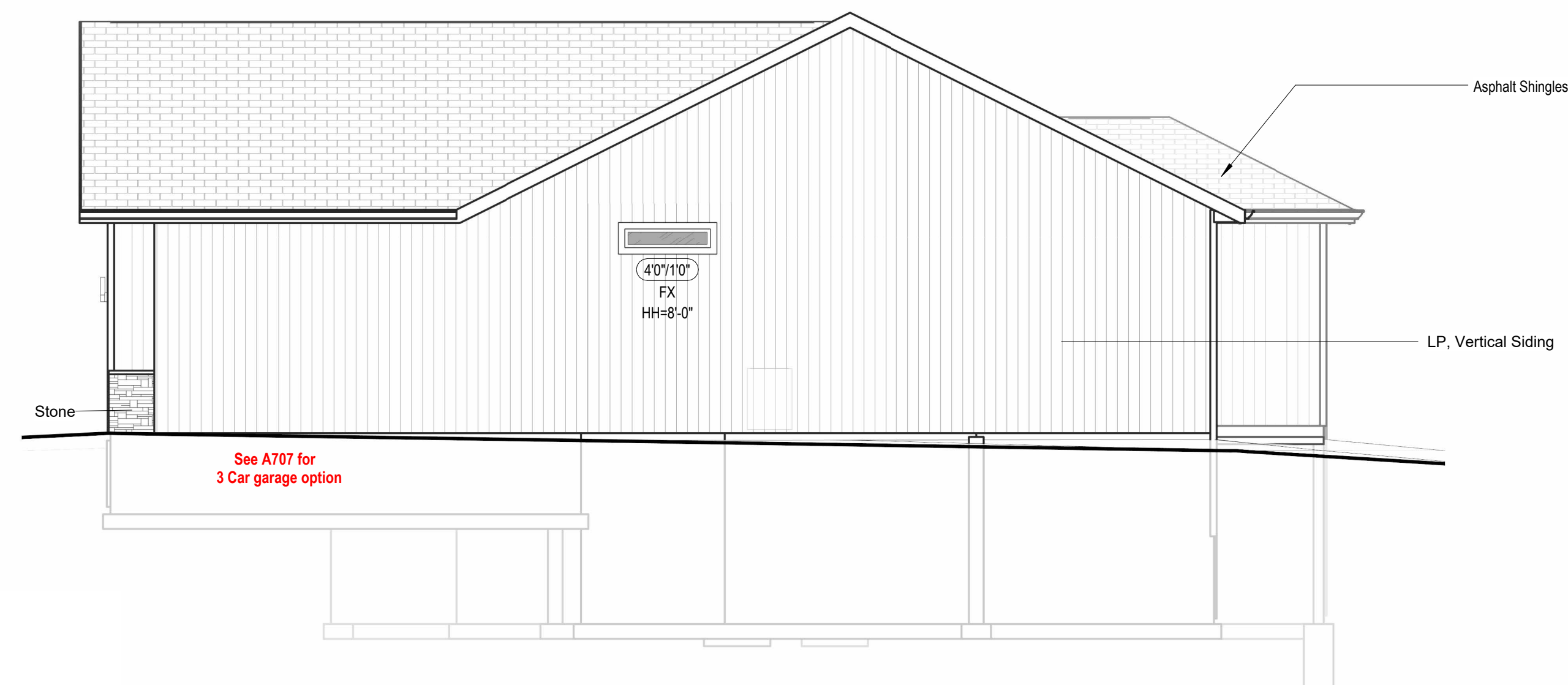
① Right Elevation - Full Basement - Farmhouse 3/16" = 1'-0"
