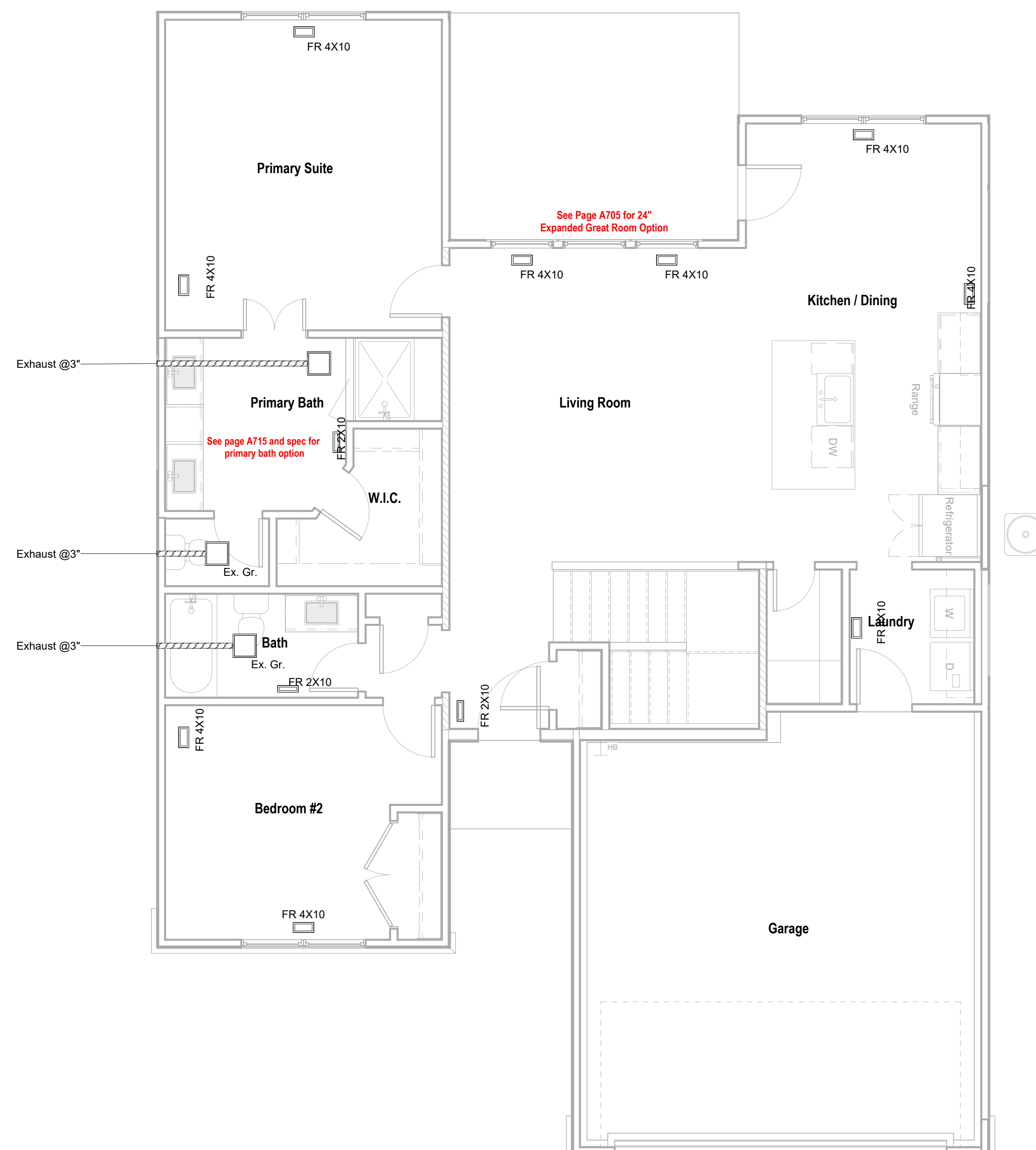
② Main Level Plan HVAC 1/4" = 1'-0"
