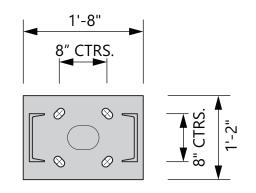
BASE PLATE DETAIL SCALE - 3/4" = 1'- 0"
