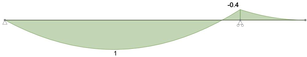
Strength combinations - Moment envelope (kip_ft)
