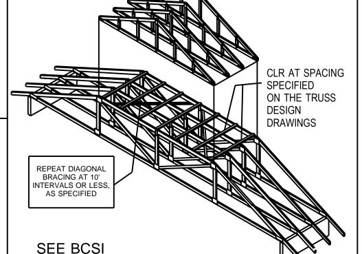
AND DIAGONAL BRACING REQUIRED SEE TRUSS DESIGN DRAWINGS FOR LATERAL RESTRAINT; CONSULT A BUILDING DESIGNER AND/OR BCSI-B3 FOR ADDITIONAL BRACING RECOMMENDATIONS
