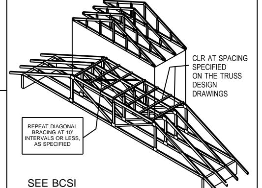
PERMANENT LATERAL RESTRAINT AND DIAGONAL BRACING REQUIRED
